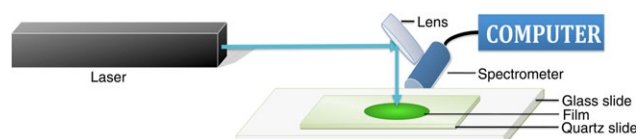
Figure 1. Fluorescence spectroscopy set-up for the film study. [Color figure can be viewed in the online issue, which is available at www.interscience.wiley.com .]
